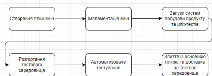
Fig. 4. Optimized process of continuous integration and implementation of changes
